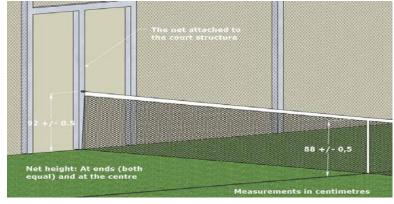
The net is suspended by a metal cable with a maximum diameter of 0.01 metres; the ends are attached to two lateral posts with a maximum height of 1.05 metres. Or a part of the court structure which allows the correct suspension and tension.
