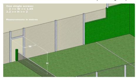
2) With two lateral accesses per side the openings must be a minimum of  $0.72 \times 2.00$  m and a maximum of  $1.00 \times 2.20$  m (See diagram).
